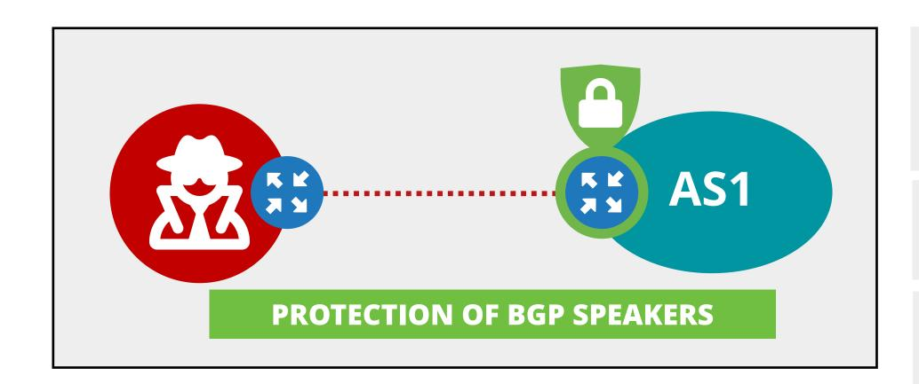
Only BGP peers to send packets to TCP 179: Control Plane Policing (CoPP), or ACLs (if CoPP not supported)
