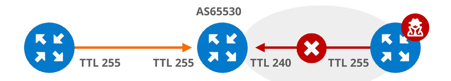
GTSM **enabled**, TTL of all BGP packets are set to 255
