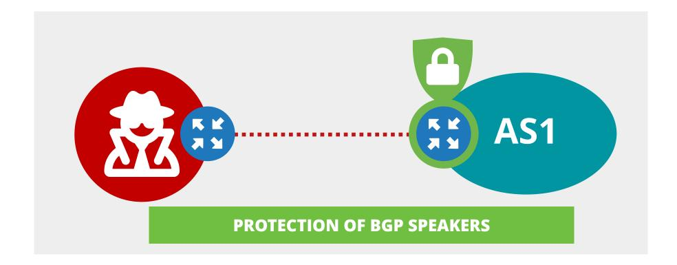
Only BGP peers to send packets to TCP 179: Control Plane Policing (CoPP) or ACLs (if CoPP not supported)
